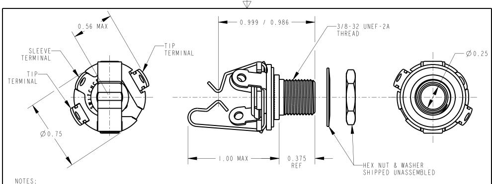
I. MATERIALS: BUSHING - COPPER ALLOY, NICKEL PLATED TIP SPRINGS - NICKEL SILVER SLEEVE TERMINAL - COPPER ALLOY, TIN PLATED INSULATING WASHERS - PHENOLIC JACK WASHER - STEEL, NICKEL PLATED HEX NUT - COPPER ALLOY, NICKEL PLATED MOUNTING WASHER - STEEL, NICKEL PLATED
