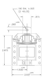
Solenoid shown energized in drawing with plunger fully seated
