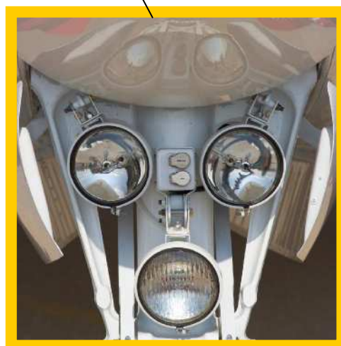
LANDING GEAR LAMPS
