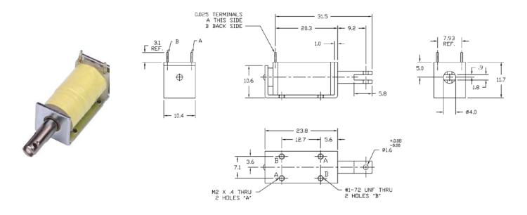
Solenoid shown energized with plunger fully seated
